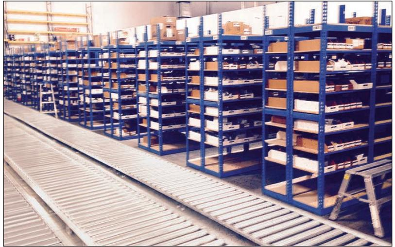
WPSS’ Southwest regional sales manager, Scott Hebert, pointed out that the RiveTier product contributes to the profits of its installers, by reducing installation costs by 30-40% over bolted shelving. With its boltless connections, assembly is quicker, easier and RiveTier has no small parts to misplace.
