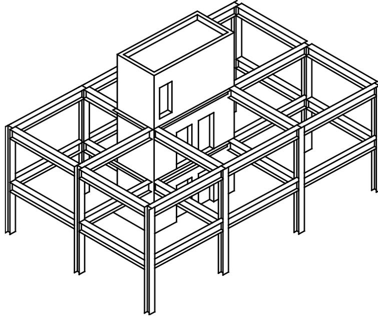
**Figure 3.** Steel Frame With Shear Wall.
