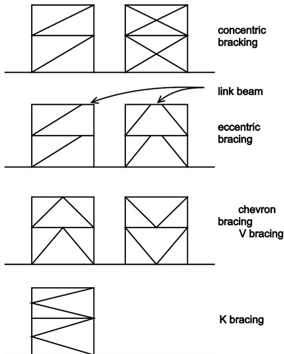
**Figure 4.** Bracing Types.
