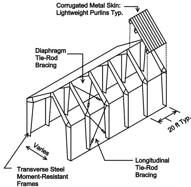
**Figure 6.** Light Metal Construction.
