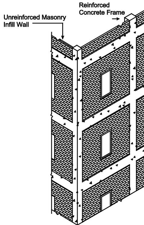
**Figure 5.** Concrete Frame With URM Infill.
